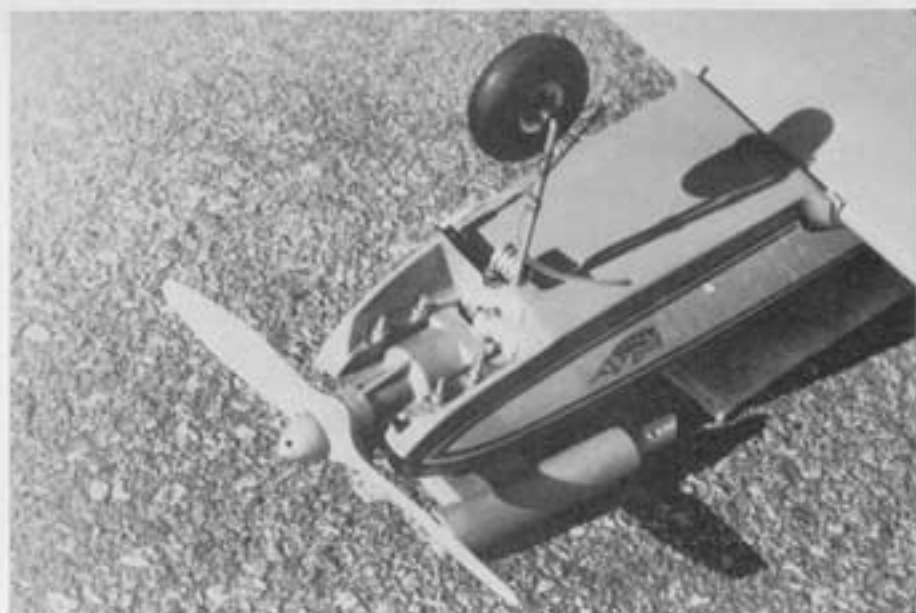
Open area in nose section for steering and engine mounting allows easy access for repairs or changes.
