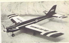
The latest version of the Blue Angel shows an even shorter nose, with a deeper profile to accommodate retract, the absence of any wing fences and a redrafted vertical tail.
