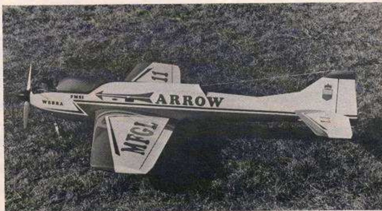
Deep fuselage houses tuned pipe. Probably helps knife-edge flight, too.
