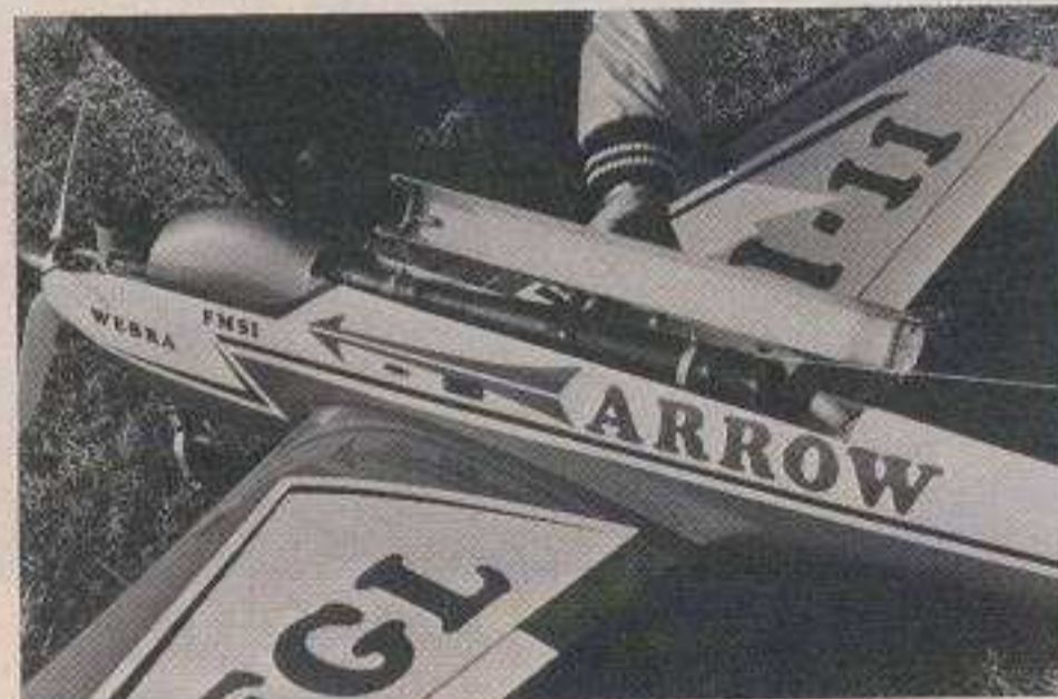
Tuned pipe is housed on top, exhaust ducted out bottom.
